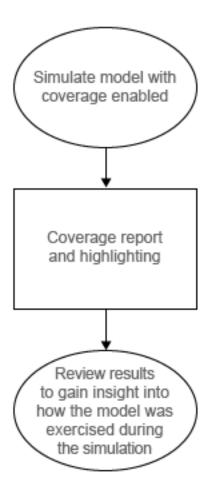
After you enable coverage for a model with test cases, Simulink Coverage reports on, and highlights in the model, those objects in your design that were exercised during simulation. You use the coverage reports and model highlighting to learn which parts of your model were active during the specified test cases.
